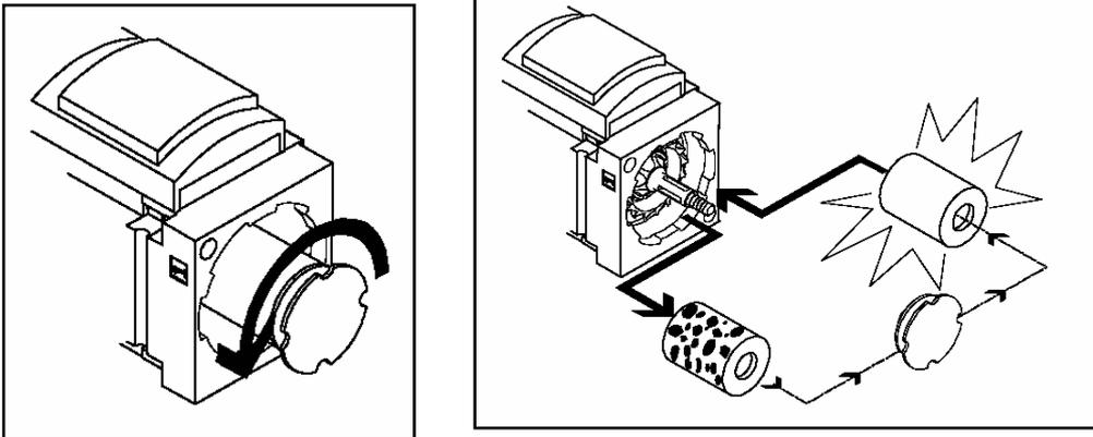
Fasten the filter screw and place the filter bowl back . Make sure the locking pin points towards the large recess.
